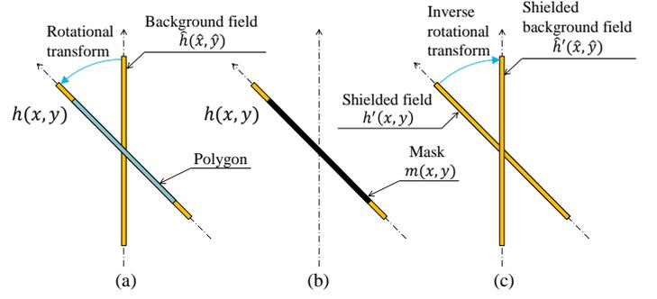
Figure 1. The procedure for rigorous light-shielding.
