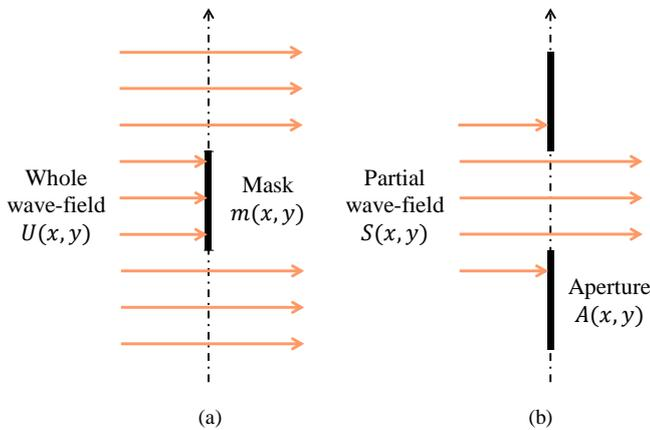
**Figure 4.** Light-shielding by the mask (a) and aperture (b). These can be equivalent to each other by using Babinet's principle and a partial field propagation [11]
