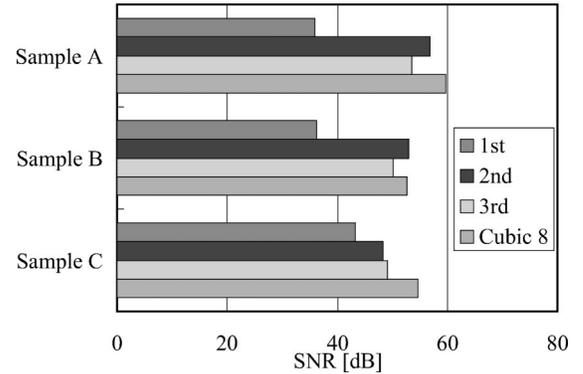
Fig. 6. SNRs in one-dimensional amplitudes for several interpolation algorithms. Here  $n$ th and Cubic 8 stand for  $n$ th iterative linear interpolation and cubic interpolation at 8 points, respectively. The rotation angle is  $30^\circ$ .
