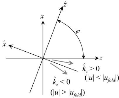
Fig. 10. Schematic depiction of the spectral fold. Each side with respect to the maximum or minimum value in frequency transformation curves corresponds to the sign of the  $\hat{k}_z$  element of wave vectors in the reference coordinates.
