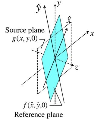
Fig. 1. Definition of source and reference planes
