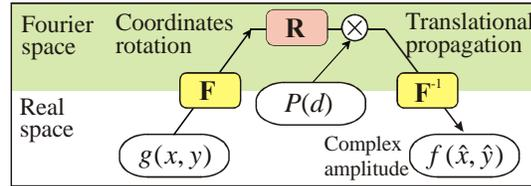
Fig. 6. Numerical procedure for polygon source of light
