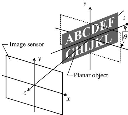
Fig. 2. Geometry for recording and numerical reconstruction of tilted planar object
