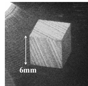
Fig. 8. Optical reconstruction of CGH created by polygon light sources
