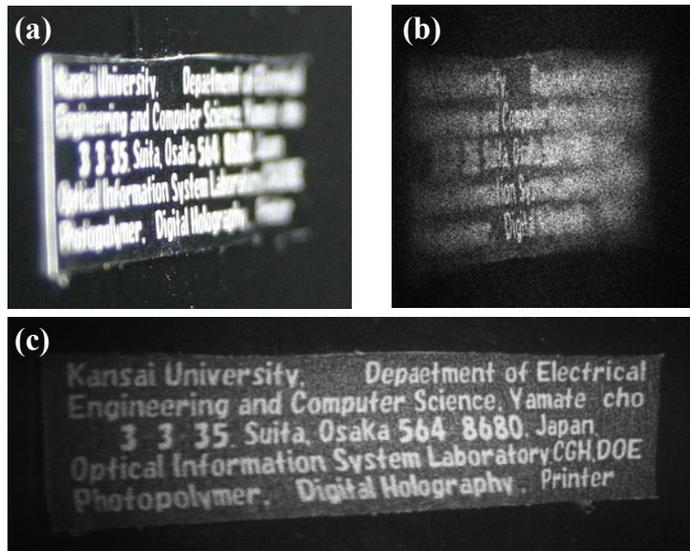
Fig. 4. Photograph of object (a), its numerical reconstruction without (b) and with (c) rotational transformation
