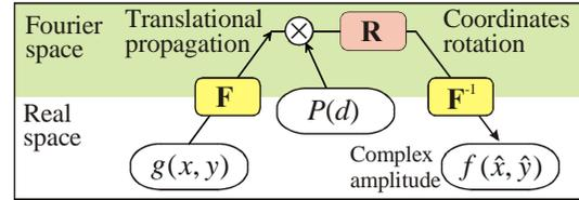
Fig. 3. Numerical procedure for reconstruction of tilted planar object
