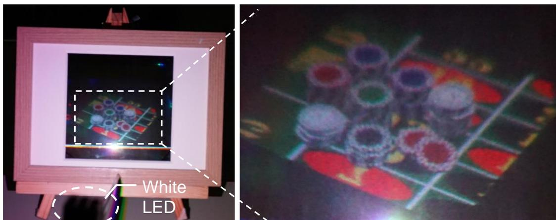
Fig.4 Optical reconstruction of a HD-CGH named 'Casino Chips'.
