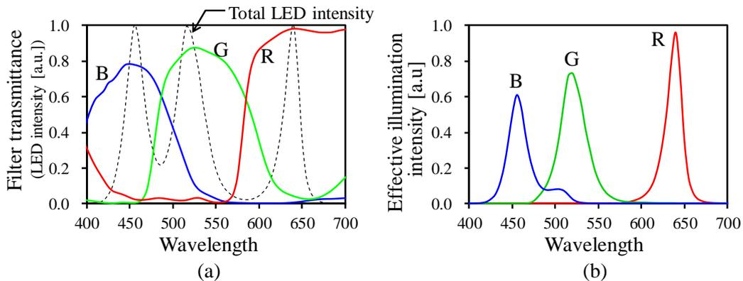
Fig.3 Spectra of (a) transmission of the fabricated RGB filter and (b) effective illumination estimated by the white LED spectrum used for the light source.
