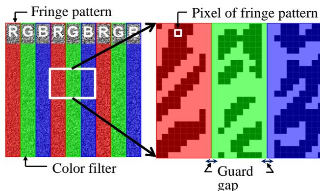
Fig.2 Color filters attached to the fringe pattern with guard gaps.
