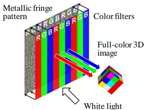
Fig.1 The principle of full-color CGH using RGB filters.
