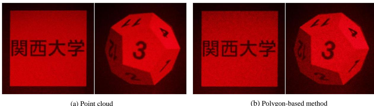
Fig. 2 Pictures of optical reconstruction of CGHs calculated by using (a) point cloud and (b) the polygon based method.
