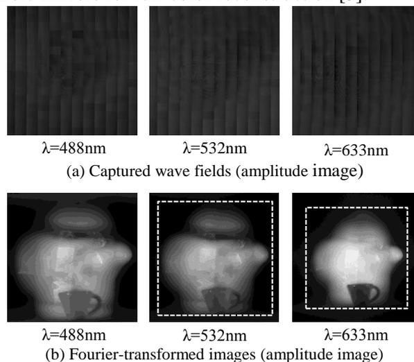
Fig.2 Captured object fields with three wavelengths
